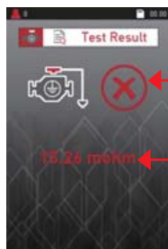
Test result indicating the ground connection is not good.
